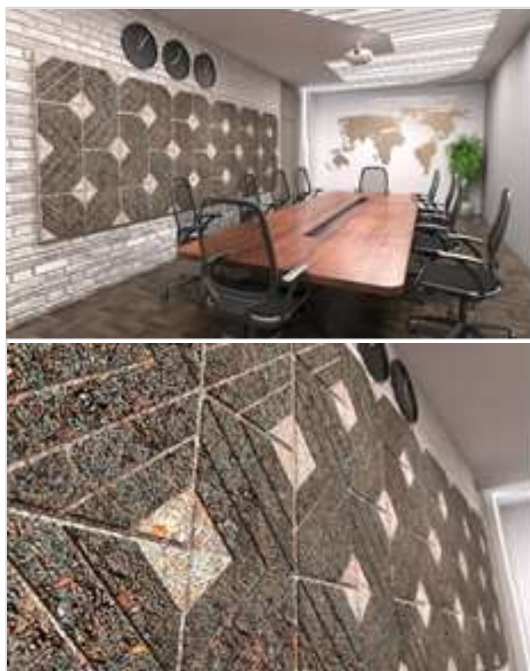
Figure 6. Soundproofing design recommendation from tea grounds
