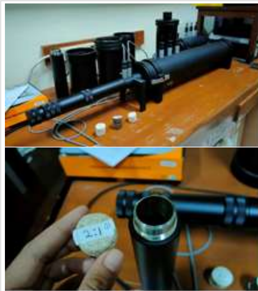
Figure 2. Instrumen and samples for sound absorption test with reference to ASTM E-1050-98
